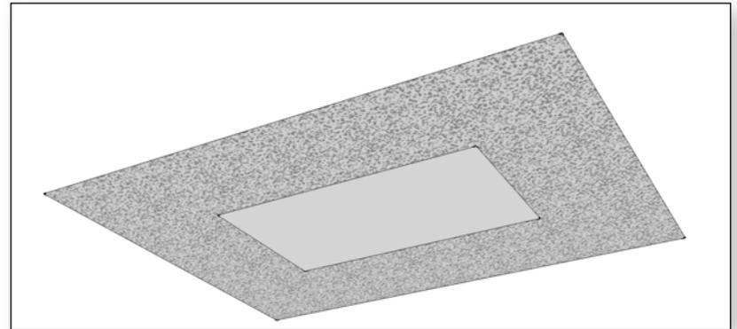
Proprietary acoustic tiles (usually 12" square, but can be larger) with an NRC value of 0.50 to 0.75 are usually the most cost-effective solution, and can be fixed to the ceiling with special adhesive. They are most effective when left unpainted, as the paint tends to reduce their sound absorptive properties.
