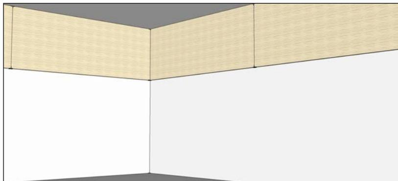
If a more architectural look is preferred, consider a system making use of spaced wood boards such as solid wood or a particle-board type product. They can be cut into slats of various dimensions, and installed on spacers away from the actual wall surface.
