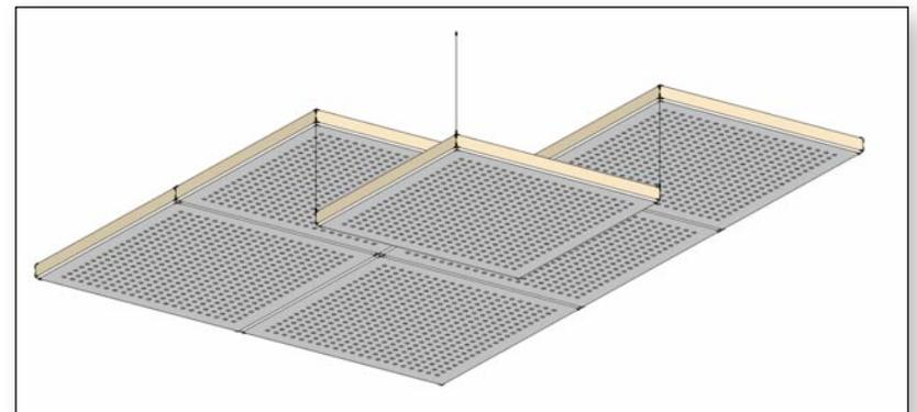
In certain situations suspended elements can be introduced into the classroom. These need to be of sound absorbent materials, and are usually hung at a high level from the ceiling. Care should be taken in their placement to avoid conflicts with lights and air diffusers.
